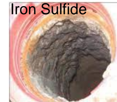
(a) Scale deposited in downhole tubular
