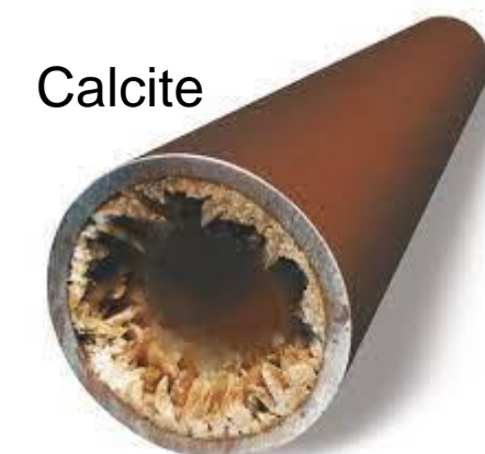
(a) Scale deposited in downhole tubular
